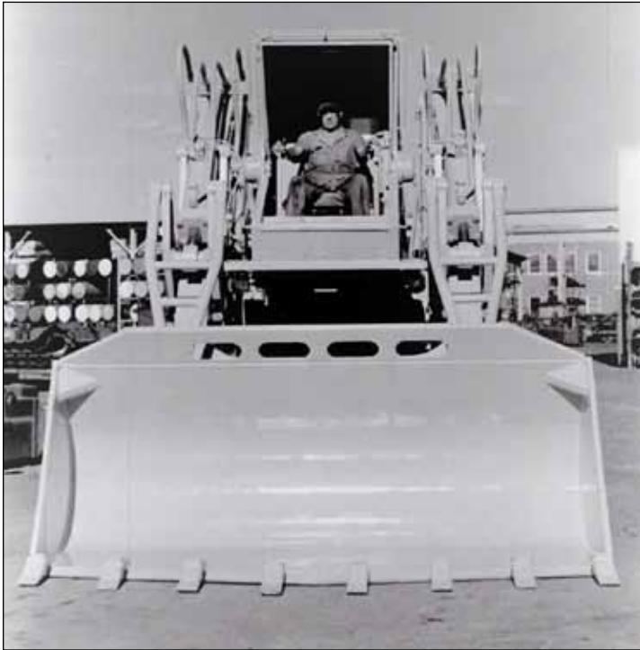
The “High Centered” Operators Cab
